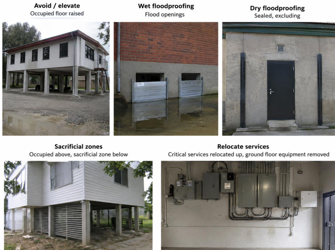
Figure 7.5 Elevation and floodproofing strategies
