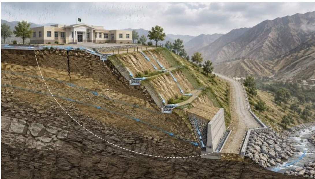
Figure 9.2 Slope cross-section: ground model features and design cases
