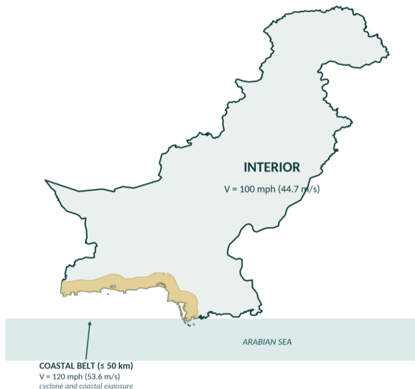
Figure 8.1 Basic design wind speed regions (schematic; design values per BCP-2021 §1609.3)
