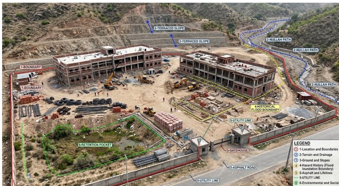
Figure 5.1 Site evidence read on an example plan
