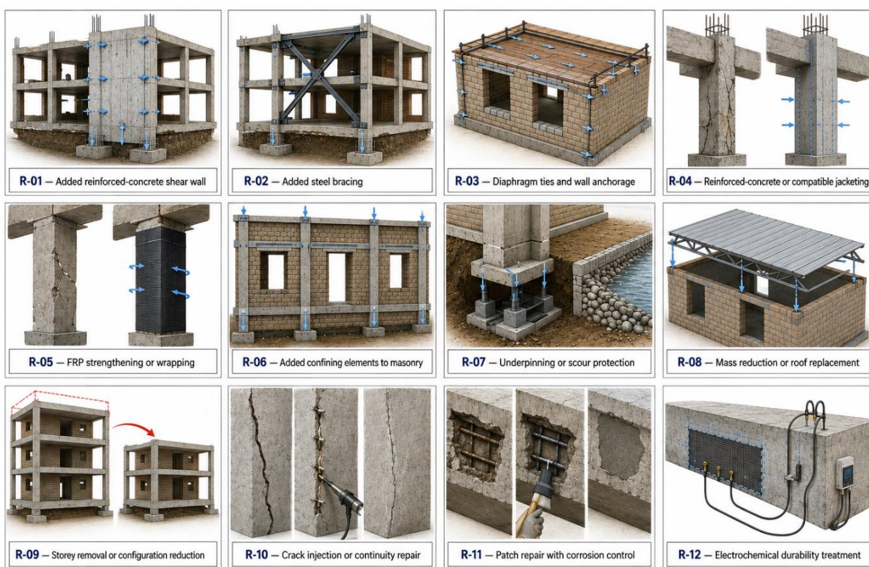
Figure 13.1 Conceptual overview of the canonical R-01 to R-12 retrofit-technique families
