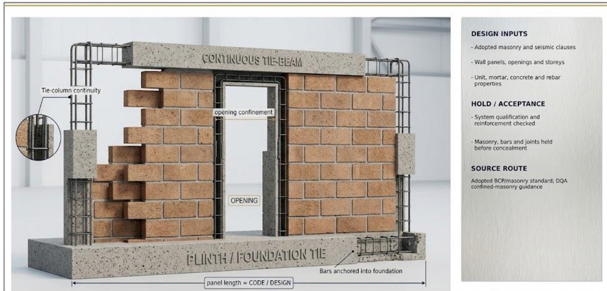
Figure 14.2 D-02: Confined masonry tie-column and tie-beam system
