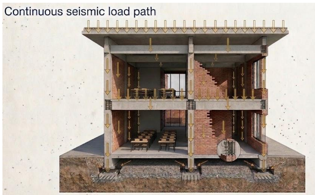
Figure 6.1 Continuous seismic load path
