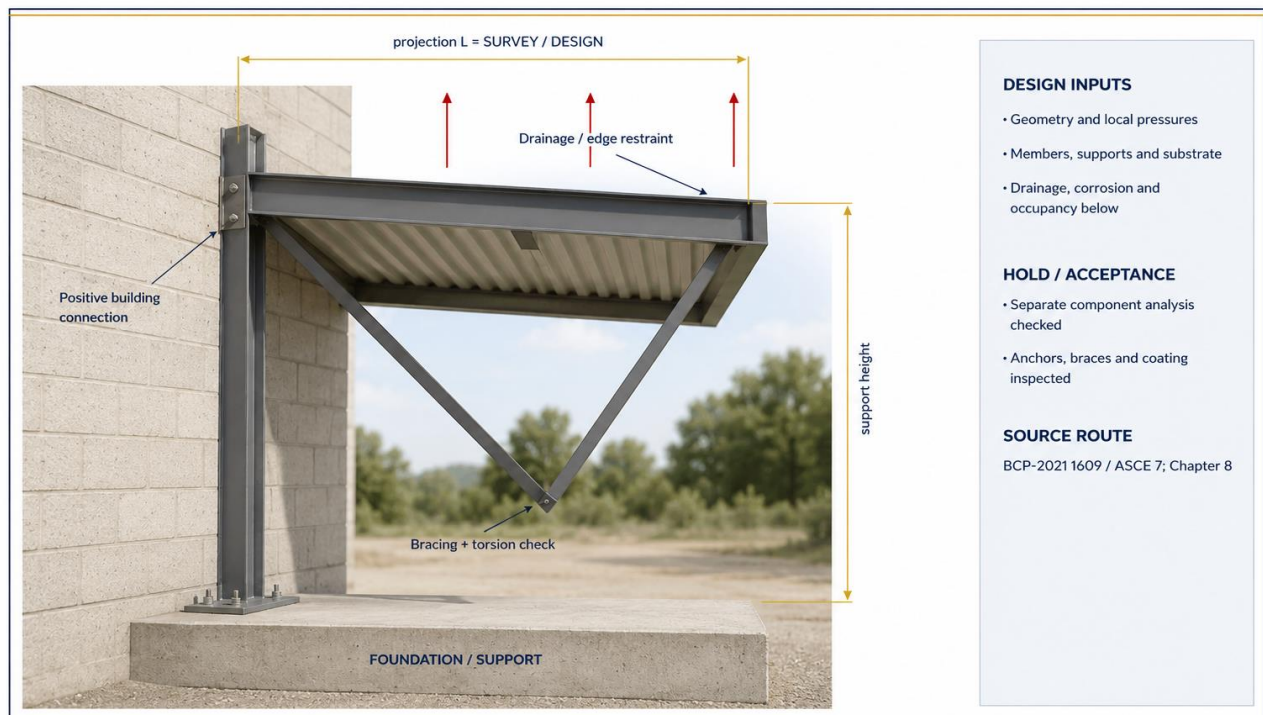
Figure 14.15 D-15: Verandah, canopy and overhang bracing
