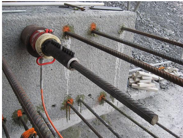
Figure 15.1 Anchor proof testing (illustrative, digitally generated; not a project record)
